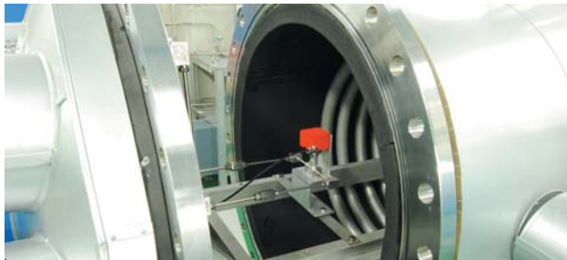
Inside the explosion-resistant chamber
