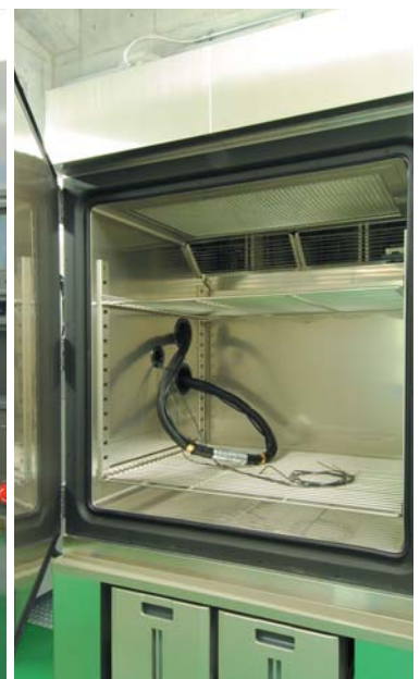
Inside the environmental test equipment
