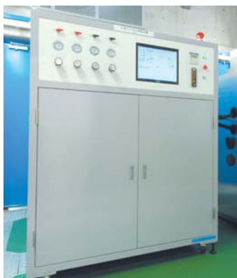
Hydrogen property preparation system
